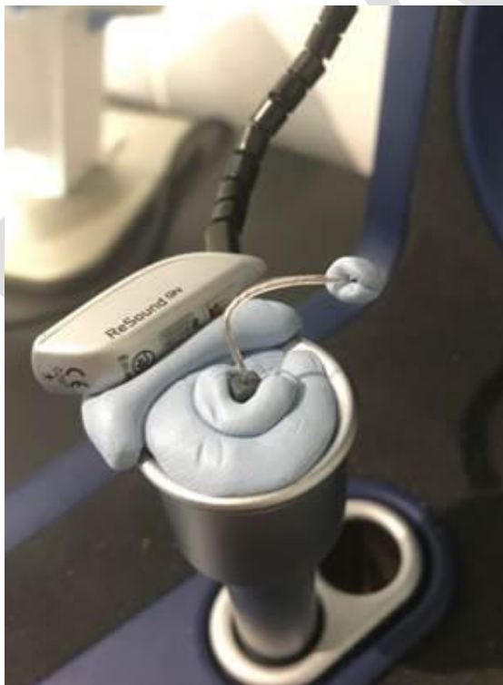
495 Figure 3: Using putty to replicate the dampening effect of the tubing sitting against a hearing 496 aid wearers head.
