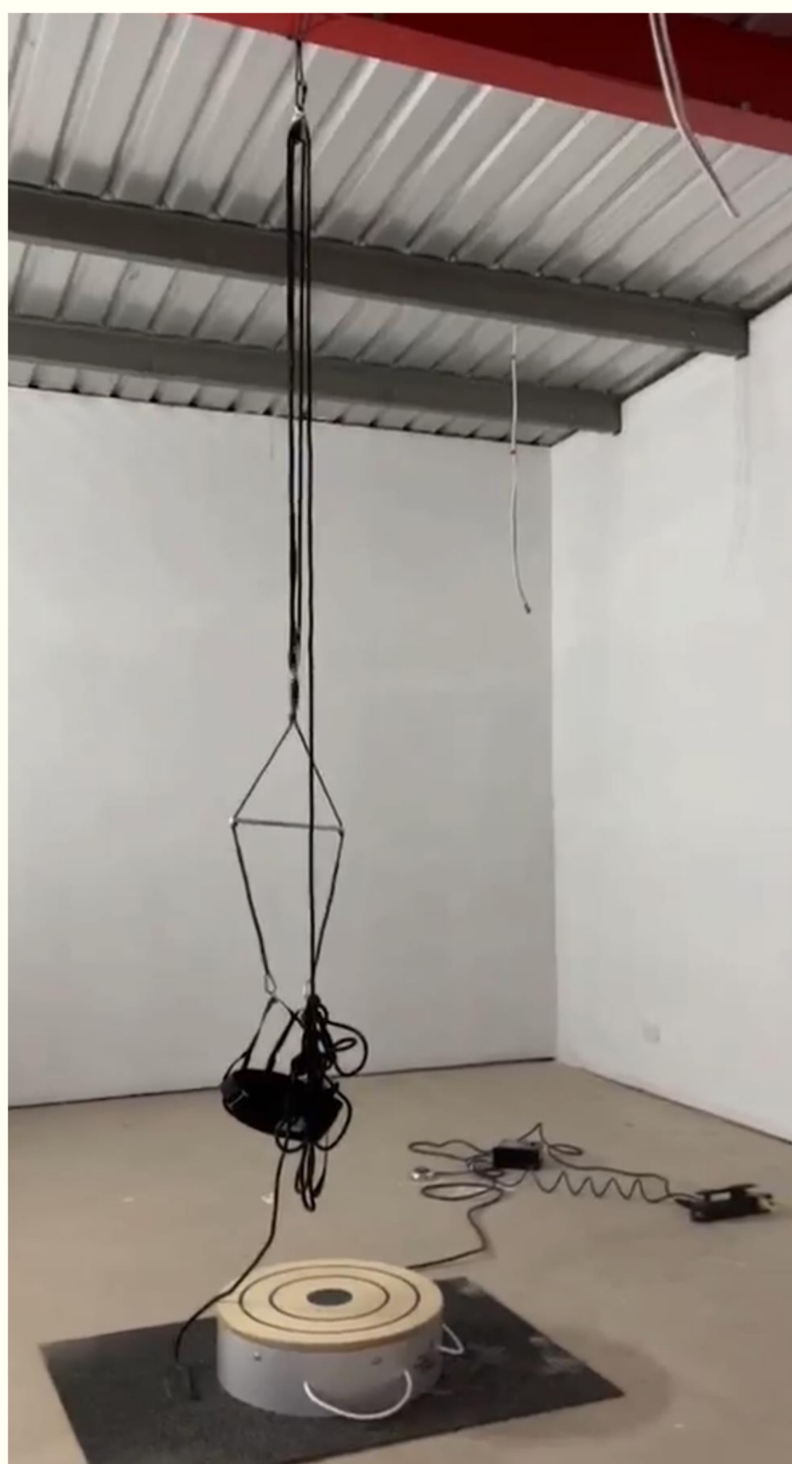
Motorised Rotational Platform and Harness Setup With permission of Sheila Thelan, Vestibular Training Services
